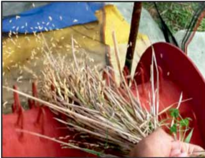
The thresher separates the grains from the stalks
