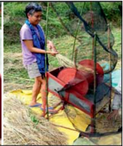
The thresher separates the grains from the stalks
